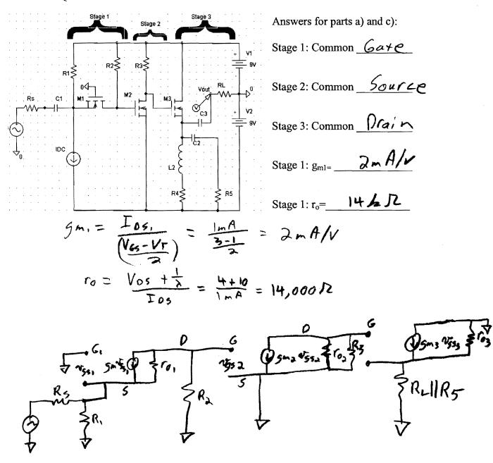
**<u>13</u>** (20-points) Given the following circuit, a) (15 points) what is the AC voltage gain,  $V_{out}/V_{in}$ ? b) (5 points) What is the input resistance? SHOW ALL WORK TO GET CREDIT!!!!!
