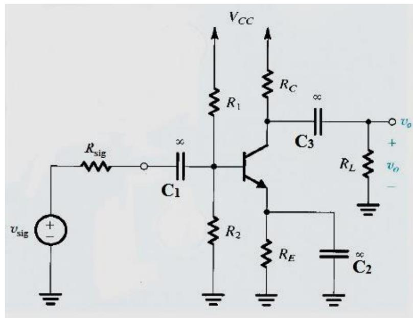
Figure 1. BJT amplifier circuit.
