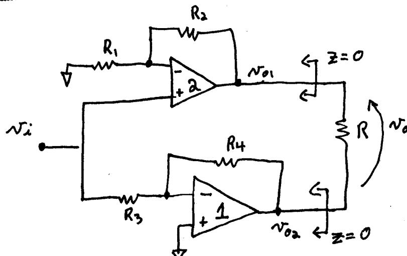
Zero output impedance allows us to decouple the stages 1+2
