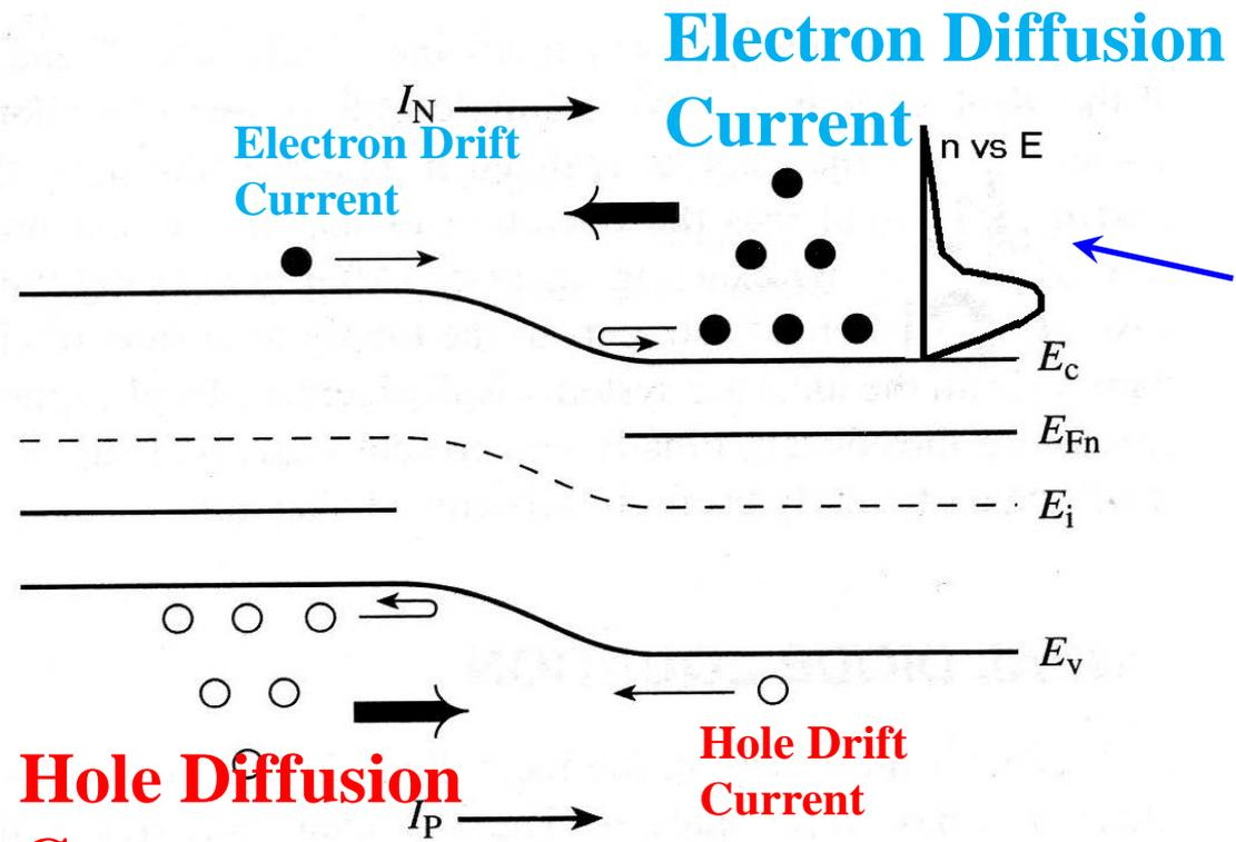
Current flow is proportional to  $e^{(V_A/V_{ref})}$  due to the exponential decay of carriers into the majority carrier bands
