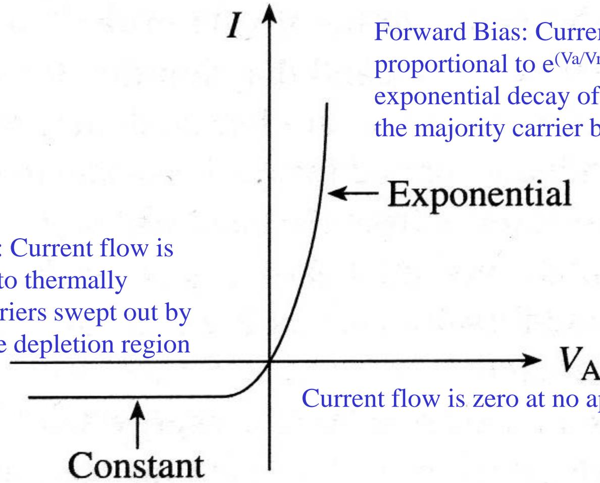
Forward Bias: Current flow is proportional to  $e^{(V_A/V_{ref})}$  due to the exponential decay of carriers into the majority carrier bands
