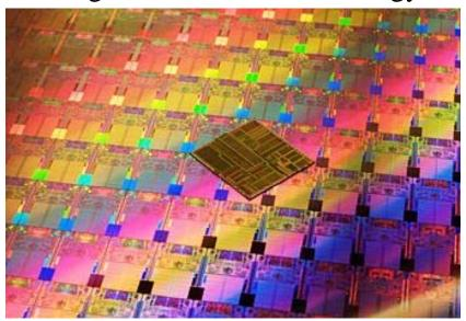
Intel, 45-nm CMOS "Dual Core" process technology Compared to older Pentium processor
