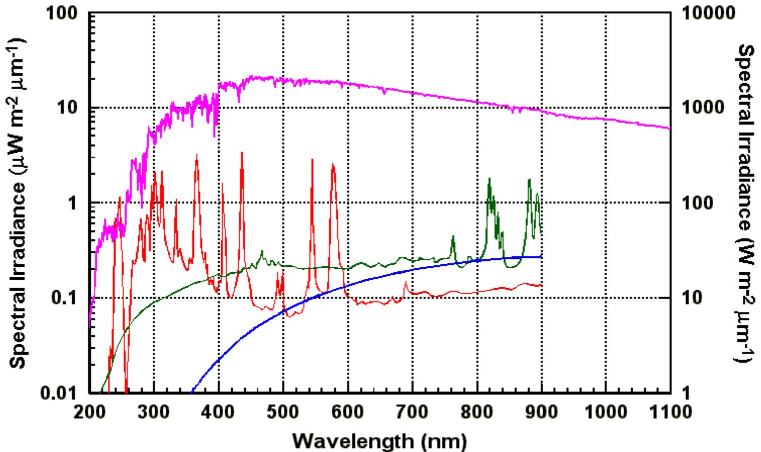
The spectral irradiance of xenon (green), halogen (blue) and mercury (red) light bulbs (left axis) are compared to the spectral irradiance from the sun (purple, which corresponds to the right axis).
