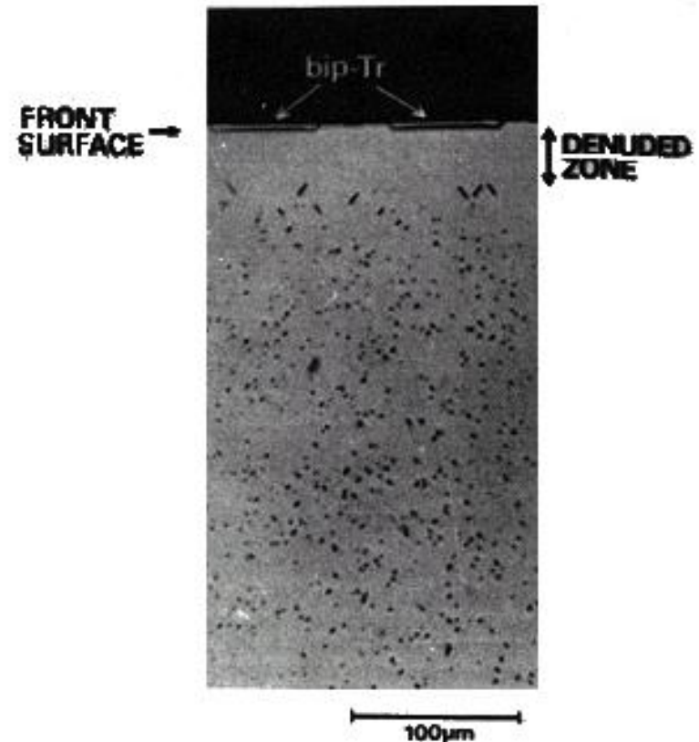
Figure 2-11 Cross section view of denuded wafer with bipolar transistor ( reprinted by permission, Academic Press, after Shimura ).
