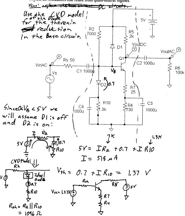
0= 1.37 - IB(1096) -0.7 - (B+1) IB (R7+R4) IB = 8.66 MA VB = V+L - IB R+L = 1.36 V Ic= 866 MA V = 5V-ICR5 = 3,27V IE = 875 MA VE = IE (RT+R4) = 0.66 V Forward Active mode is verified.
