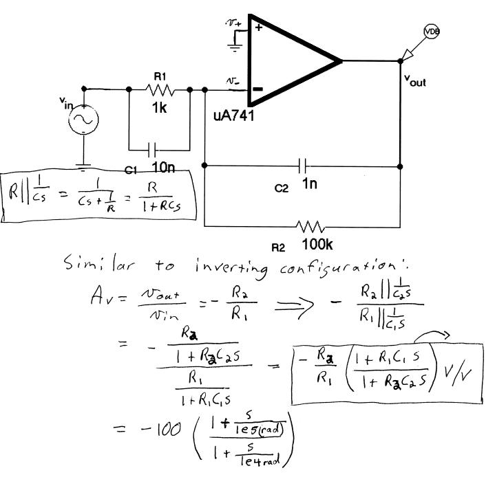
In put Impedance to the virtual ground at the Due terminal, vx (2) Virtual Ground  $|Rin = \frac{v_{\lambda}}{\lambda_{x}} = |R_{1}| \left| \frac{1}{c_{1}s} \right|$ Output Impedance.  $Rout = 0 ||R_2||_{C_2}$  Rout = 0
