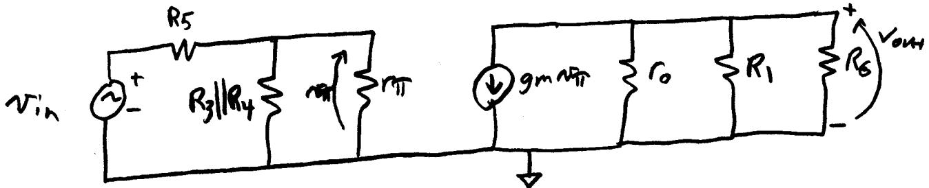
$$\frac{V_{out}}{V_{in}} = \frac{r_\pi}{V_{in}} \frac{V_{out}}{r_\pi}$$
