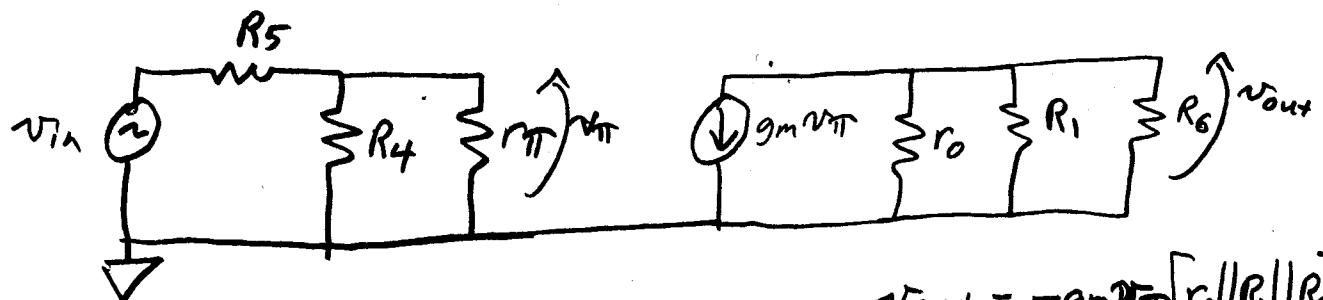
$$\frac{V_{out}}{V_{in}} = -g_m r_{\pi} [r_0 || R_1 || R_6]$$
