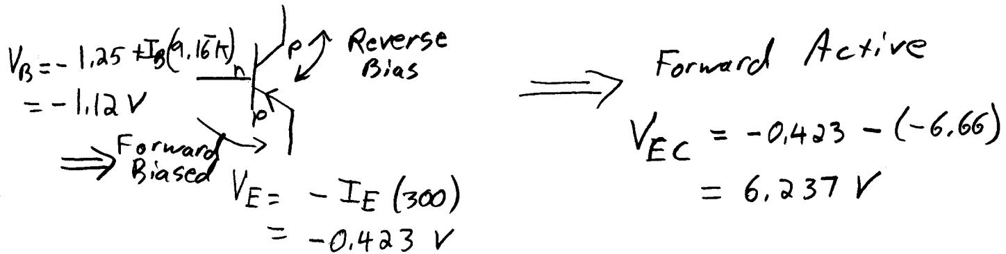
$$r_o = \frac{V_A + V_{EC}}{I_C} = \frac{75 + 6.237}{1.39 \times 10^{-3}} = 58.4 \text{ k}\Omega$$
