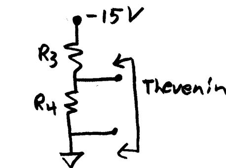
$$V_{th,base} = -15 \frac{R_4}{R_3 + R_4}$$
