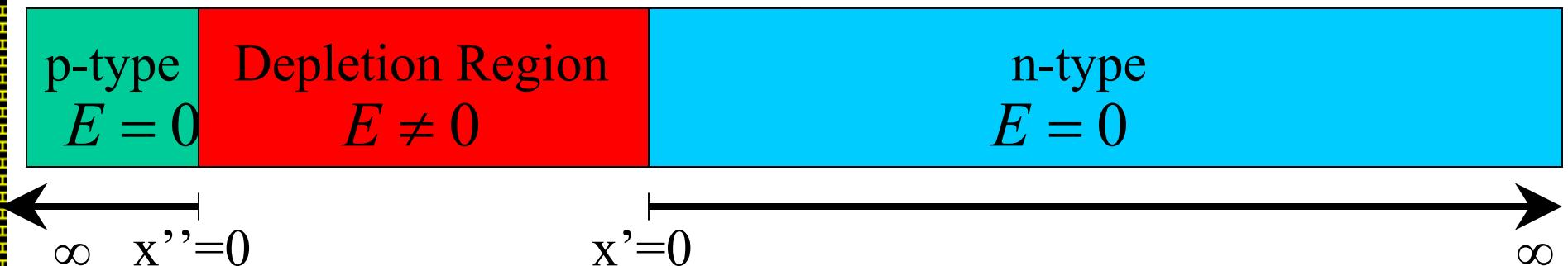
$$\Delta p_n(x') = \frac{n_i^2}{N_D} \left( e^{\frac{qV_A}{kT}} - 1 \right) e^{(-x'/L_p)} \quad \text{for } x' \geq 0$$
