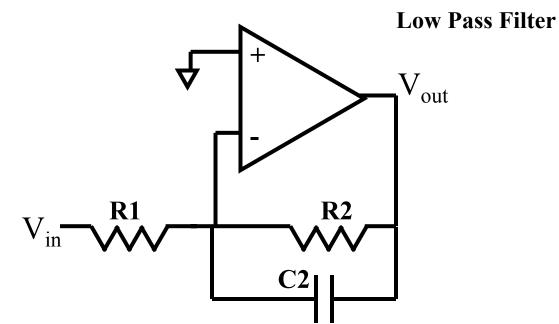
$$\frac{V_{out}}{V_{in}} = -\frac{R_2}{R_1} \left( \frac{1}{1 + R_2 C_2 s} \right)$$
