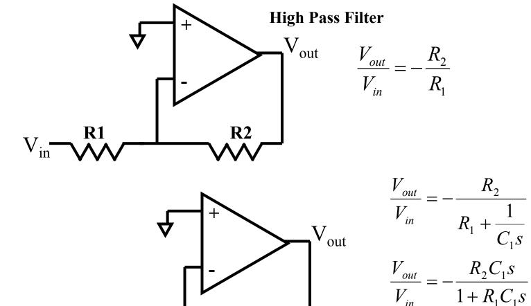
•At high frequency,  $R_1C_1s>>1$ , the gain returns to it's full value,  $(-R_2/R_1)$
