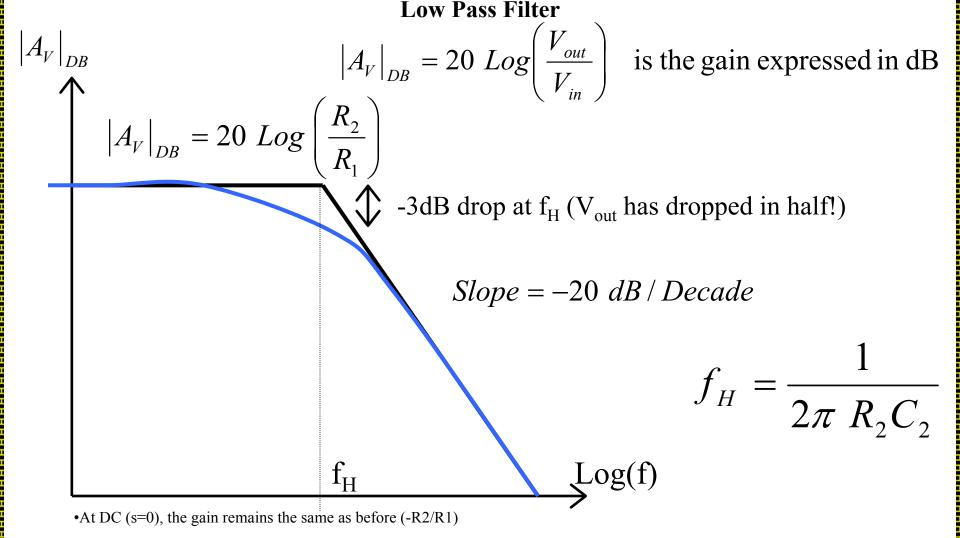
•At high frequency,  $R_2C_2s>>1$ , the gain dies off with increasing frequency
