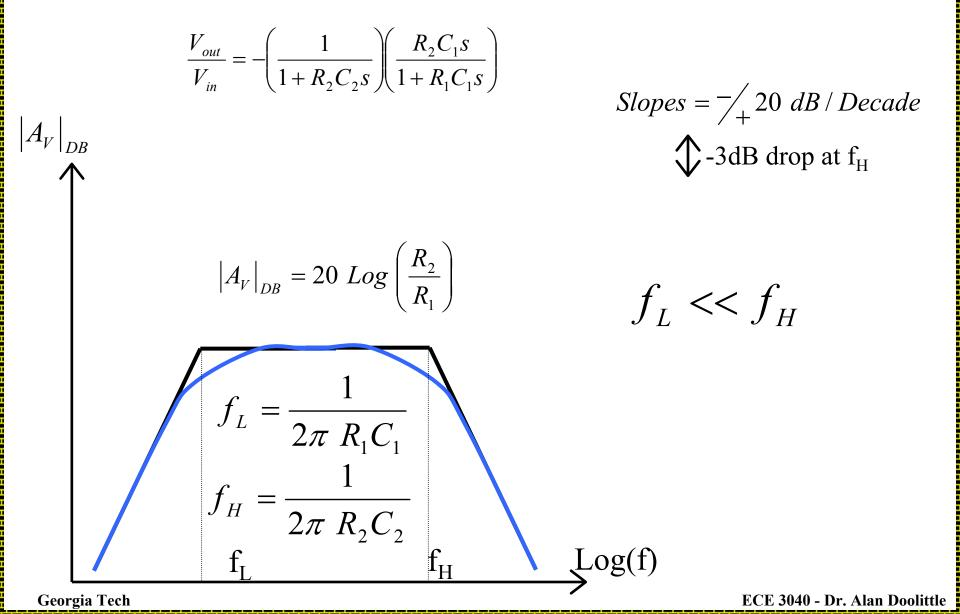
Band Pass Filter (combination of high and low pass filter)
