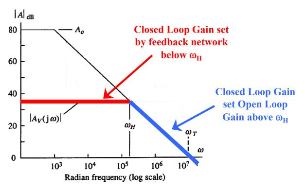
$$(Gain \ x \ Bandwidth)_{Open \ Loop} = (Gain \ x \ Bandwidth)_{Closed \ Loop}$$
