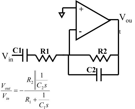
$$\frac{R_{2} \frac{1}{C_{2}s}}{R_{2} + \frac{1}{C_{2}s}} = -\left(\frac{1}{1 + R_{2}C_{2}s}\right) \left(\frac{R_{2}C_{1}s}{1 + R_{1}C_{1}s}\right)$$
