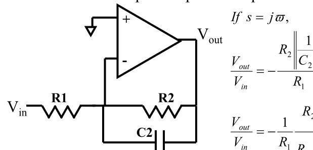
$$\frac{R_2 \left\| \frac{1}{C_2 s} \right\|}{R_1}$$
