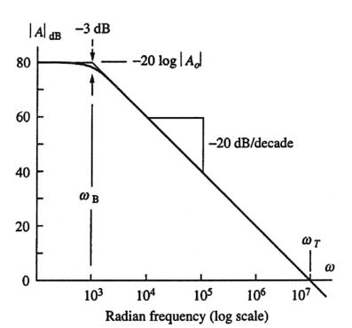
$$\left| A_{OpenLoop}(j\varpi) \right| = \frac{A_{O}\varpi_{B}}{\sqrt{\varpi^{2} + \varpi_{B}^{2}}}$$
