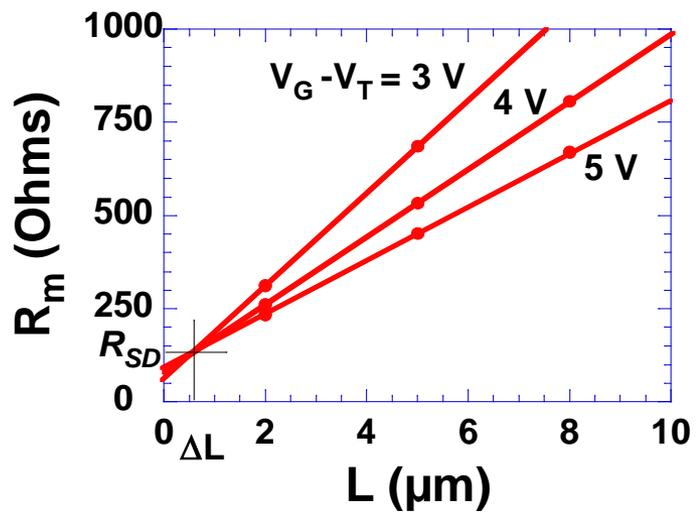
**Important Note:** you need to measure  $V_T$  of each device separately, since MOSFETs with different channel lengths have different threshold voltages!
