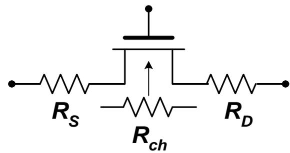
$$R_m = R_{ch} + R_{SD} = \frac{L - \Delta L}{W_{eff} \mu_{eff} C_{ox} (V_{GS} - V_T)} + R_{SD}$$
