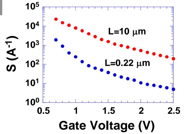
Ratio is not constant with gate voltage **ONLY** due to differences in threshold voltage.
