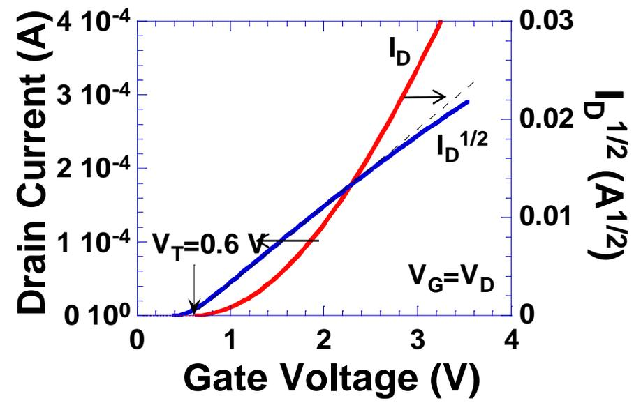
$$I_D = \frac{W_{eff} \mu_{eff} C_{ox}}{2L_{eff}} (V_G - V_T)^2$$
