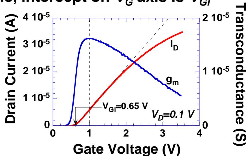
$$I_D = \frac{W_{eff} \mu_{eff} C_{ox}}{L_{eff}} (V_G - V_T - V_D/2) V_D; \quad g_m = \left. \frac{\partial I_D}{\partial V_G} \right|_{V_D = \text{constant}}$$
