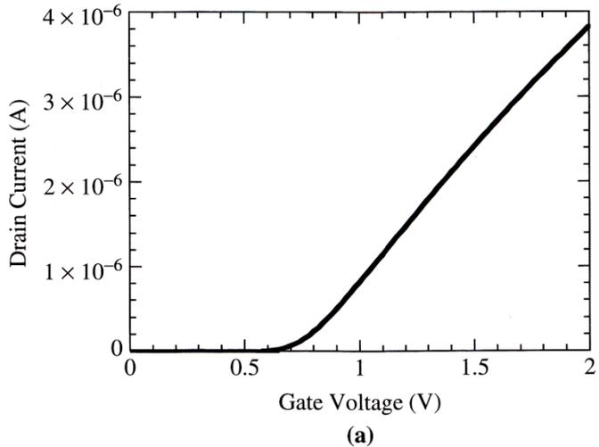
$$V_{T,2\phi_F} = V_{FB} + 2\phi_F + \frac{\sqrt{2qK_s\epsilon_0N_A(2\phi_F - V_{BS})}}{C_{ox}}$$
