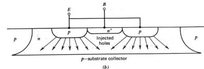
Figure 2.27b Minority-carrier flow in the substrate *pnp* transistor.
