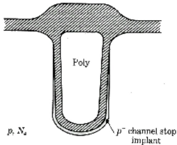
**FIGURE 5.31** Example of nonideal trench cross section.
