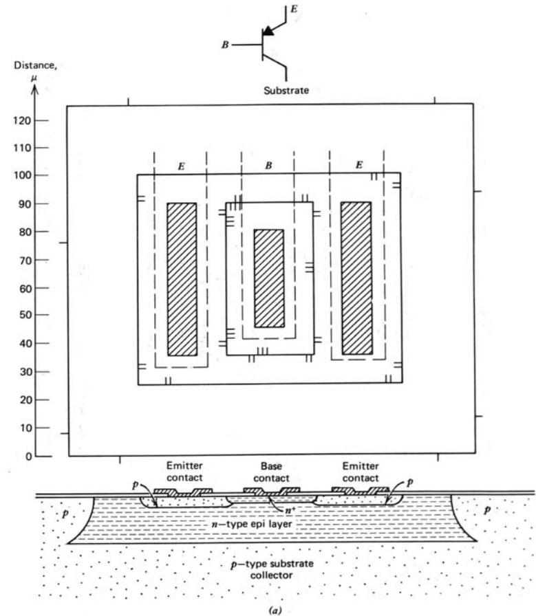
Figure 2.27a Substrate *pnp* structure.
