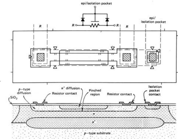
Figure 2.32 Pinch resistor structure.
