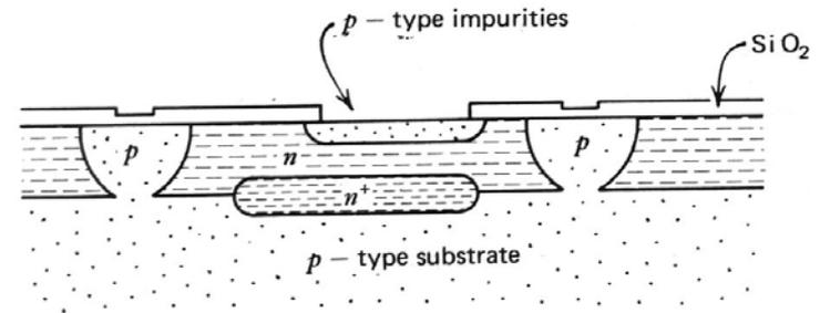
Figure 2.13 Structure following base diffusion.
