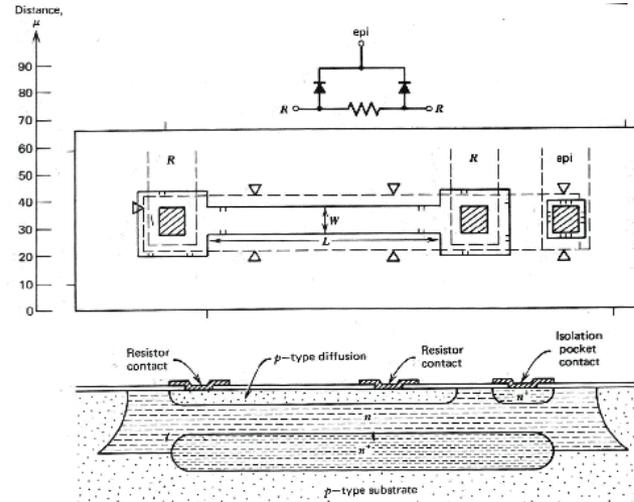
Figure 2.30 Base-diffused resistor structure.
