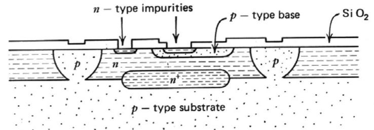
Figure 2.14 Structure following emitter diffusion.
