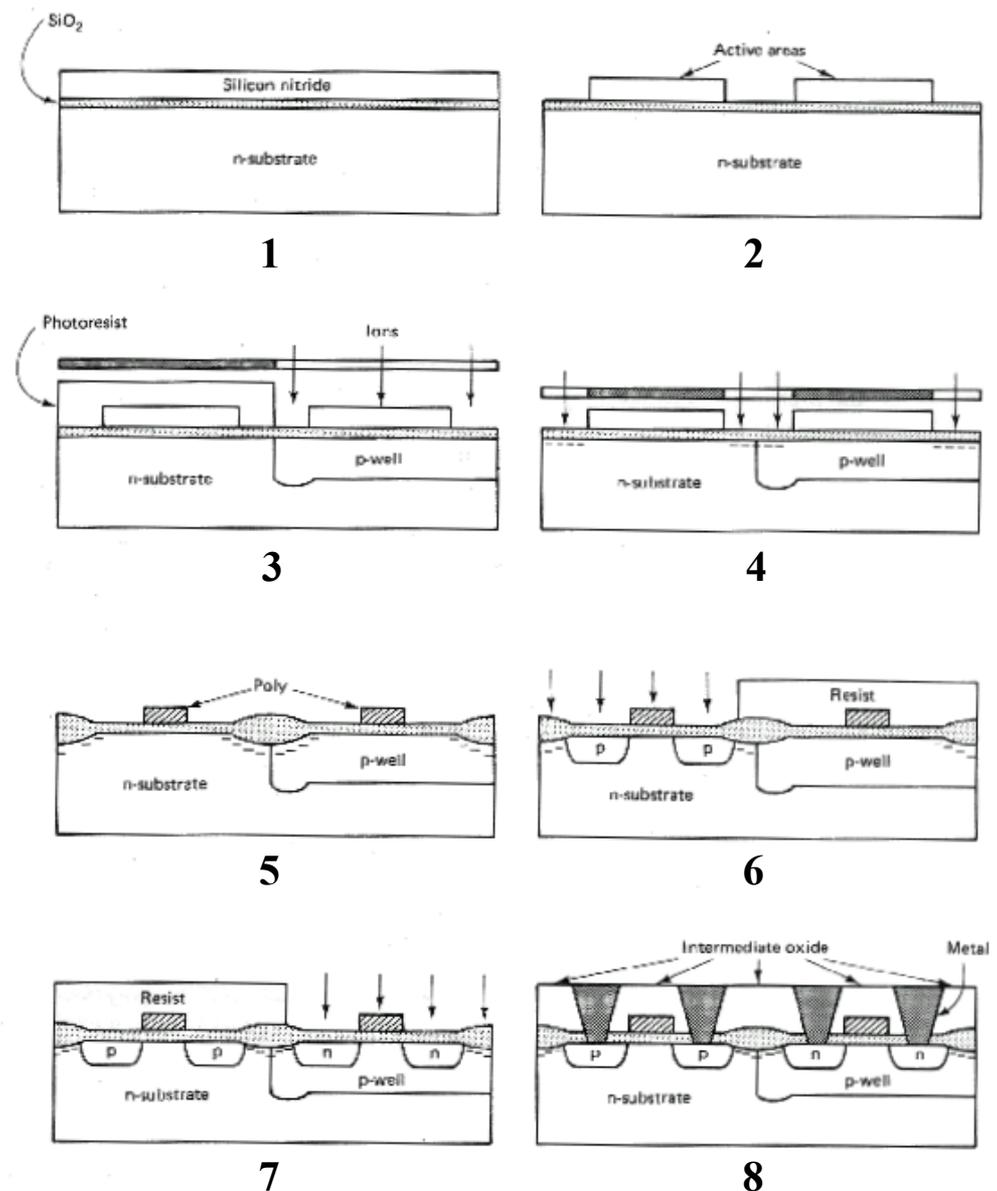
Figure 4.9 Oxide-isolation CMOS process.
