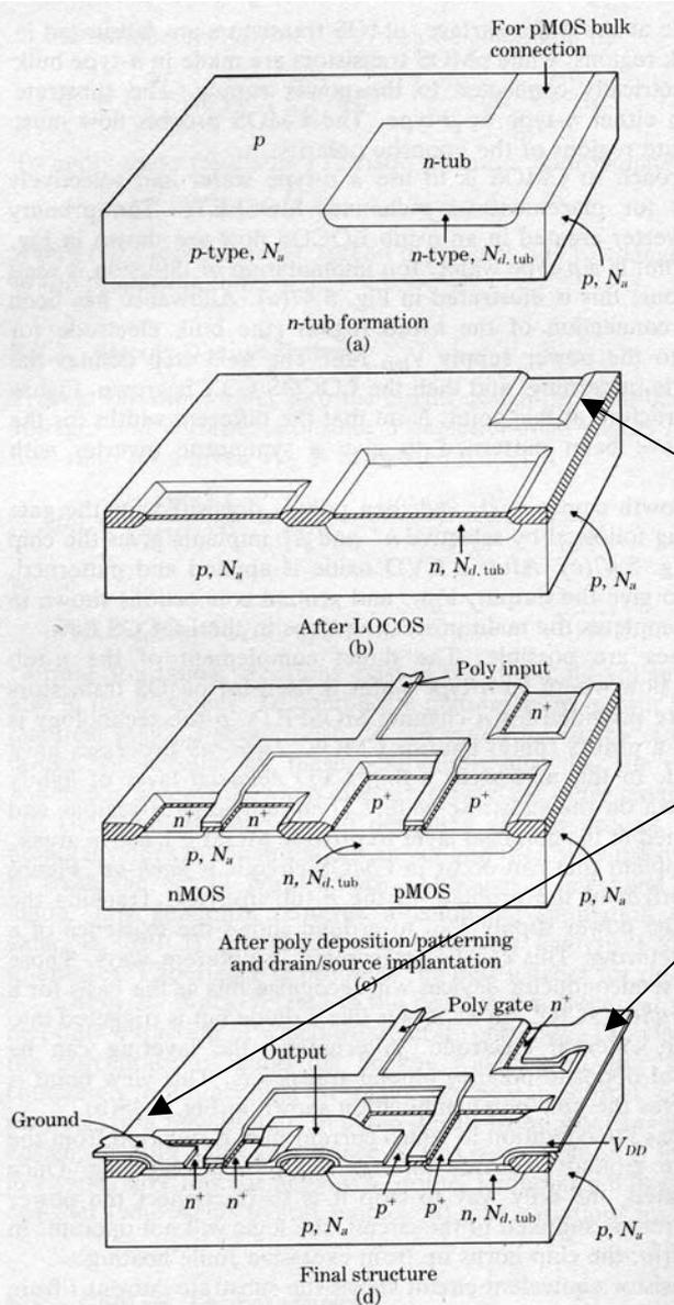
One also needs to allow for connections to properly bias the wells as shown.
