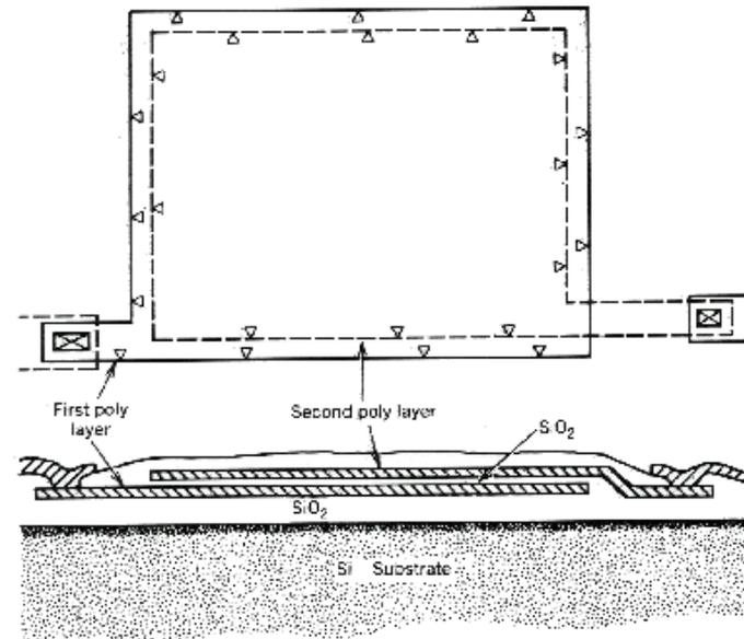
Figure 2.55b Plan view and cross section of typical poly-poly capacitor.
