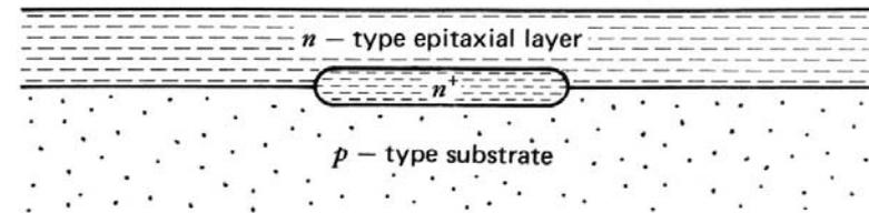
Figure 2.11 Bipolar integrated-circuit wafer following epitaxial growth.
