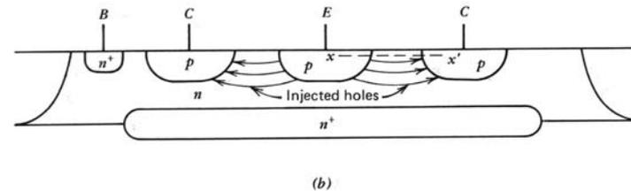
Figure 2.24b Minority-carrier flow in the lateral *pnp* transistor.
