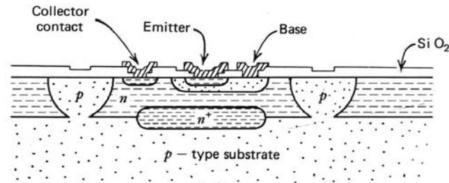
Figure 2.15 Final structure following contact mask and metallization.
