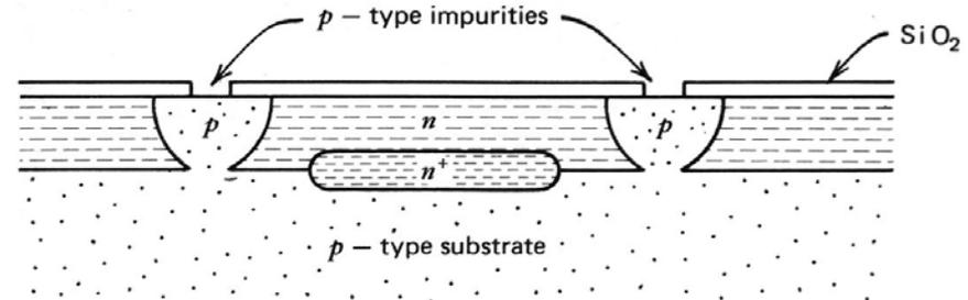
Figure 2.12 Structure following isolation diffusion.
