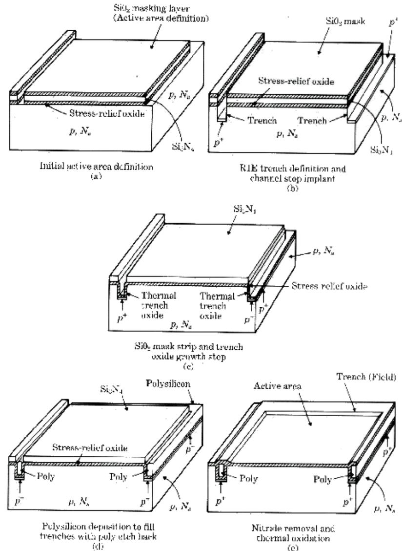
**FIGURE 5.29** Basic sequence for trench isolated integrated circuits.
