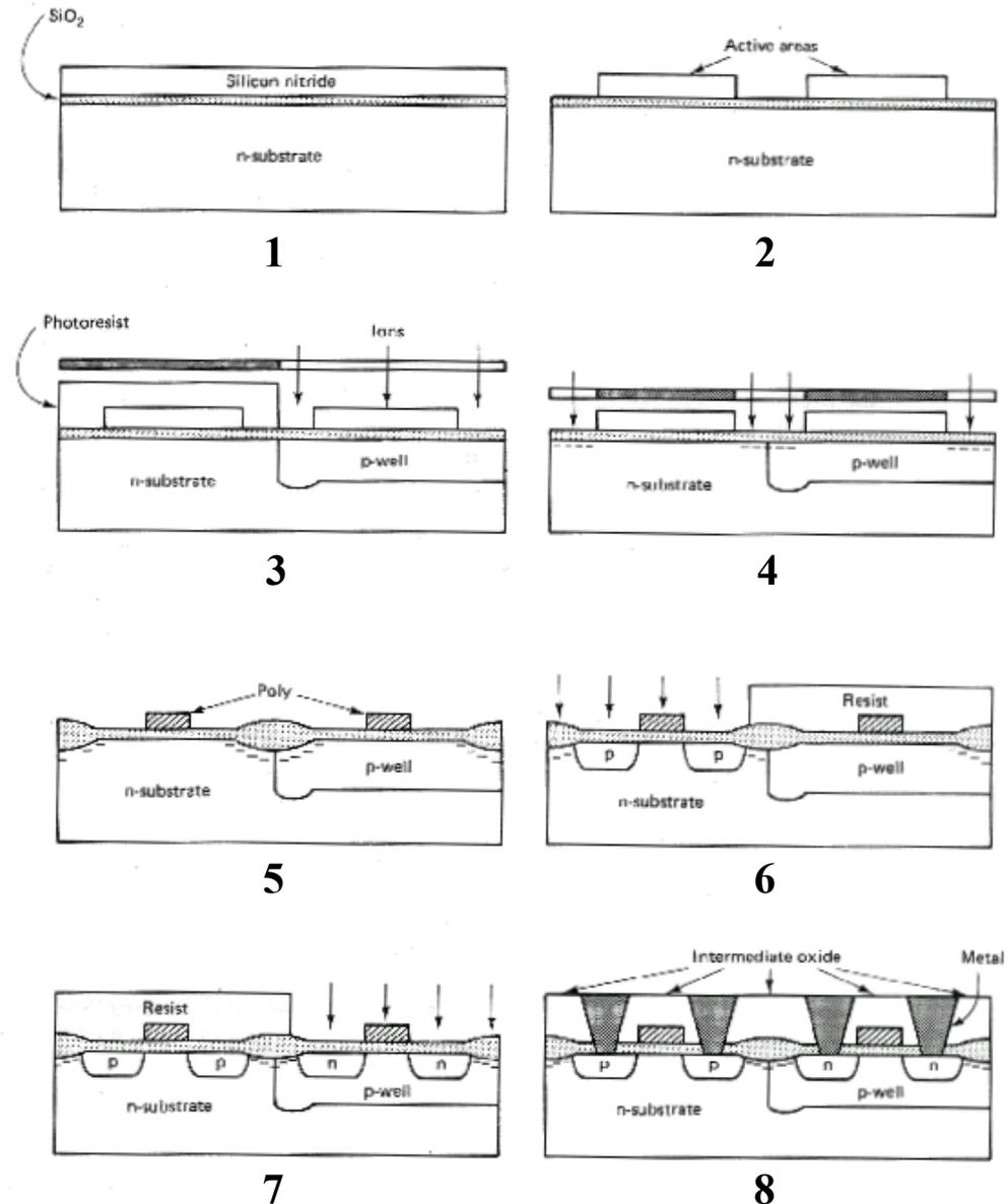
Figure 4.9 Oxide-isolation CMOS process.
