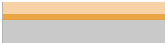
2. Coat and prebake imaging resist
